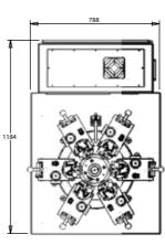
PLAN VIEW SHOWING CONFIGURATION WITH; Ø400x102 WHEEL 6-OFF STANDARD FIXTURE
